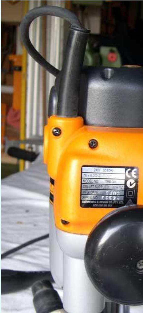
The five screws visible in this picture can be safely left alone, as they hold the switch cover assembly to the upper motor body (for completeness, they're numbers 21 and 22 in the parts diagram).
