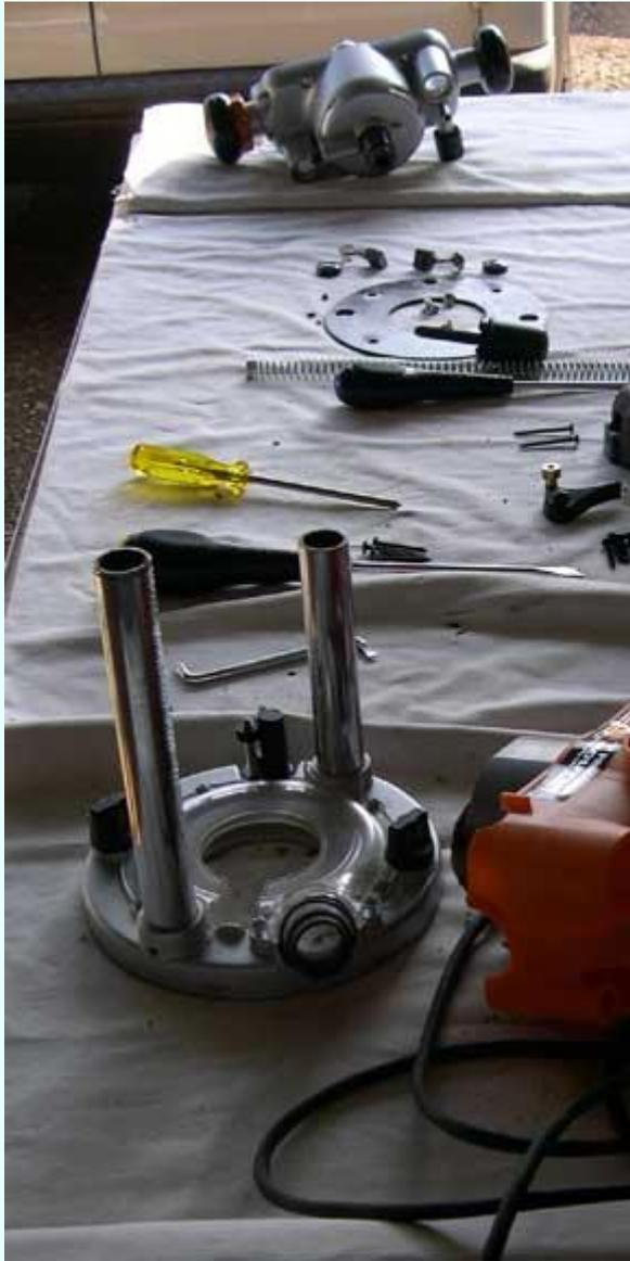
Wind the top motor body off the base unit, then separate the two halves by removing the four screws, which are now easily accessible.
