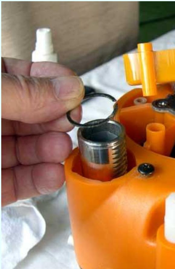
This picture shows the circlip (snap ring - 87) which must be removed from the top of the right-hand plunge tube.
