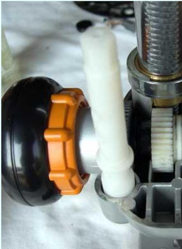
This picture shows the clutch engaged (rack-and-pinion winding mode).
